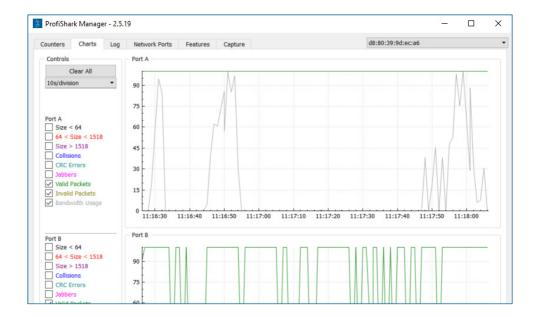
Depending on the type of packets or events selected in the left side of the screen, the statistical data is plotted accordingly for either port A or B. Refresh rate can also be selected using the drop-down list on the top left, further tuning the displayed information.
